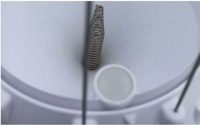
Figure 8-4. Incorrect installation: sensor is slightly offset from the triangle
