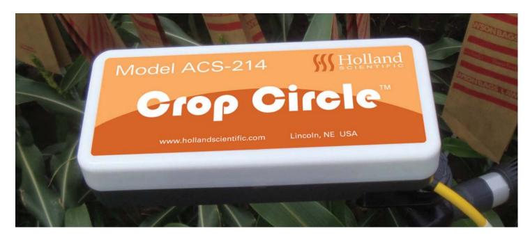
The Crop Circle ACS-214 active optical sensor (AOS) calculates the NDVI vegetation index as well as measuring canopy height via integrated radiometric, LIDAR and ultrasonic sensors.
